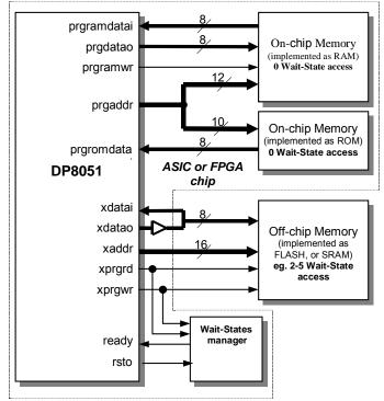
The described above implementation should be treated as an example. All Program Memory spaces are fully configurable. For timing-critical applications whole program code can be implemented as on-chip ROM and (or) RAM and executed without Wait-States, but for some other applications whole program code can be implemented as off-chip ROM or FLASH and
